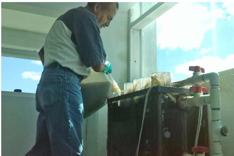
Figure 2. Inoculation of activated sludge to the aerobic reactor for biofilm production.
