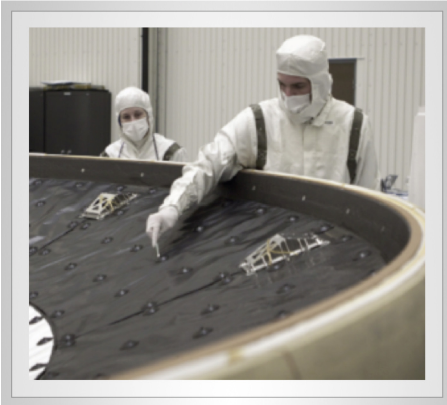
Figure 6: NASA engineers examine the heat shield of the “Curiosity Rover” and check its cleaning. Photo courtesy of NASA [6].
