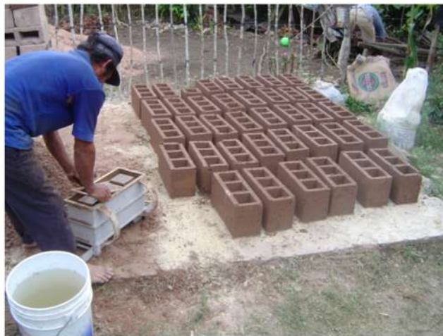
Image 6. Hollow block pieces with three cells
