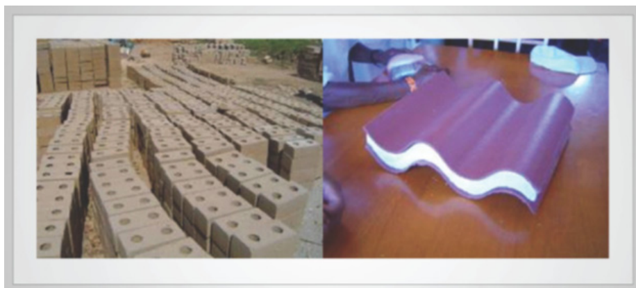
Fig. 5 Material used in the walls and roof. Blocks of improved (cement) adobe and fiber cement sheets with a 5 cm expanded polystyrene core, with the objective to reduce exterior thermal gain.
