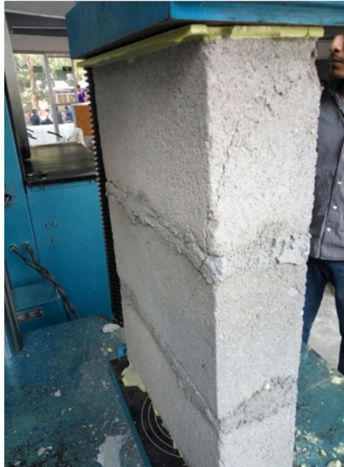
Image 4. Compression test in block piles
