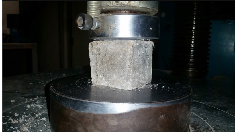
Image 1. Mortar cube test in universal press
