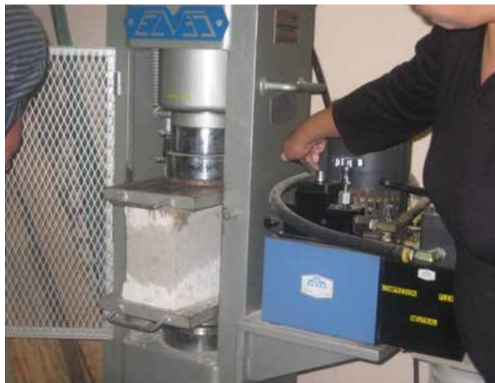
Image 14. Compression test. Source: Own elaboration
