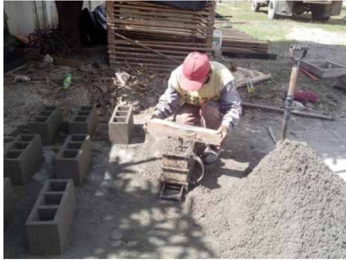
Image 16. Block manufacturing process. Source: Own elaboration
