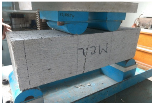
Image 11. Bending beam test. Source: Own elaboration
