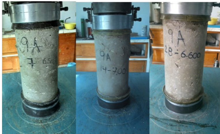
Image 10. Uniaxial compression cylinder test. Source: Own elaboration
