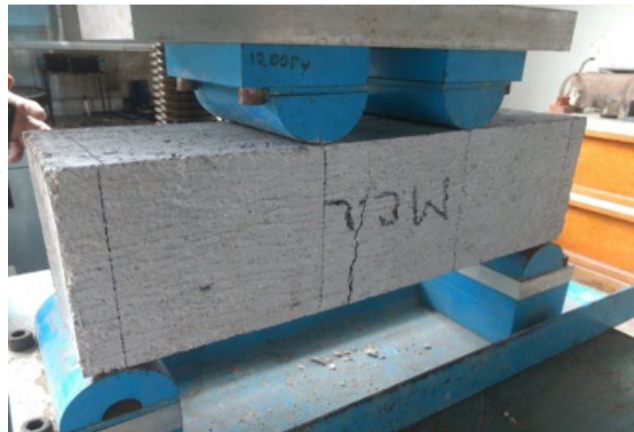
Image 11. Bending beam test. Source: Own elaboration
