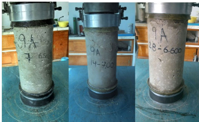
Image 10. Uniaxial compression cylinder test. Source: Own elaboration
