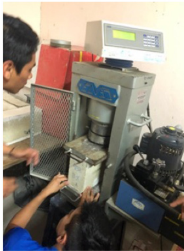
Image 1. Concrete block compression test. Source: Own elaboration
