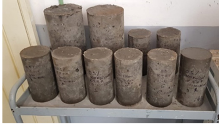
Figure 8. Cylinders with compressive strength of 24.5 MPa (250 kg/cm 2 ). Source: Image taken in the laboratory
