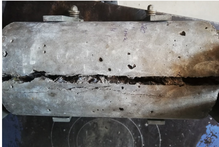
Figure 12. Tensile test failure. Source: Image taken in the laboratory
