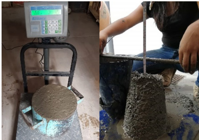
Figure 7. Density test and concrete slump. Source: Image taken in the laboratory
