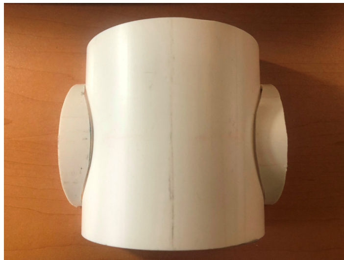
Figure 3. Model barrel vault with cropped lunettes. Source: Own elaboration
