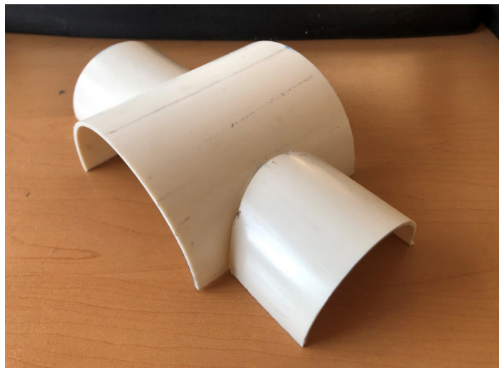
Figure 2. Model barrel vault with lunettes. Source: Own elaboration
