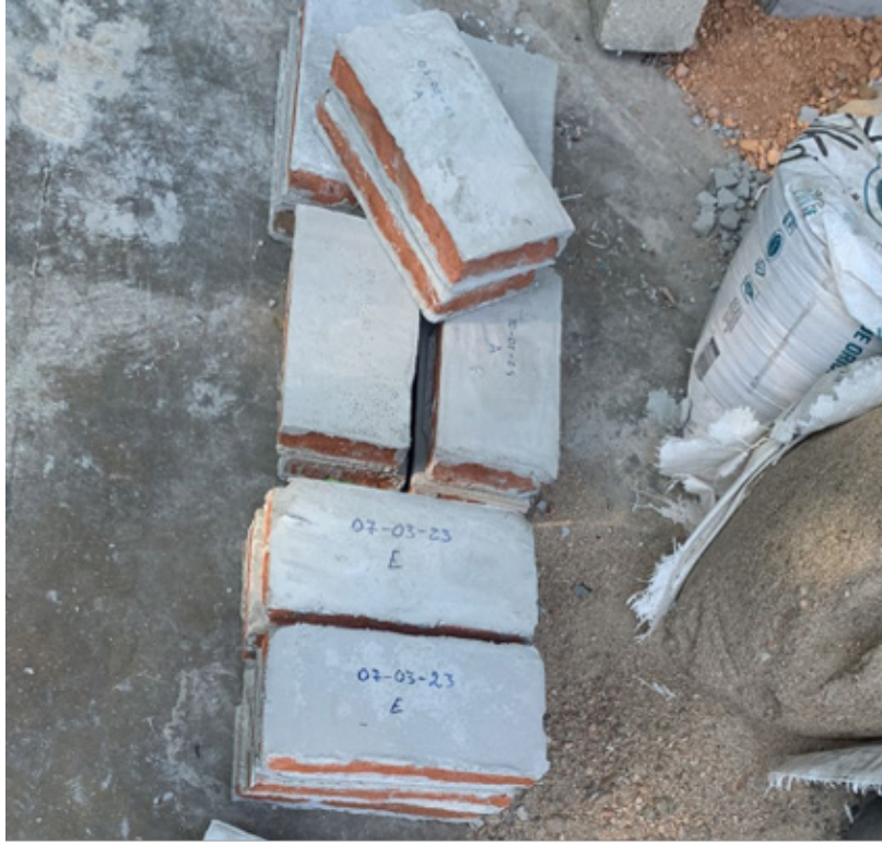
Figure 6. Pitching of the brick pieces
