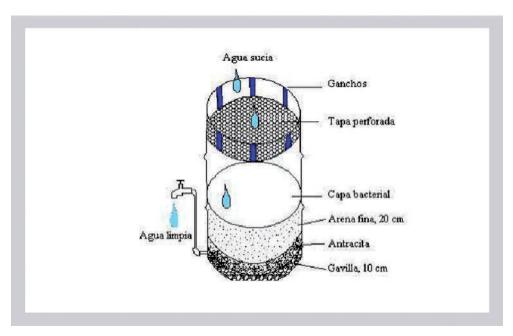
Figure 2. Homemade filter
