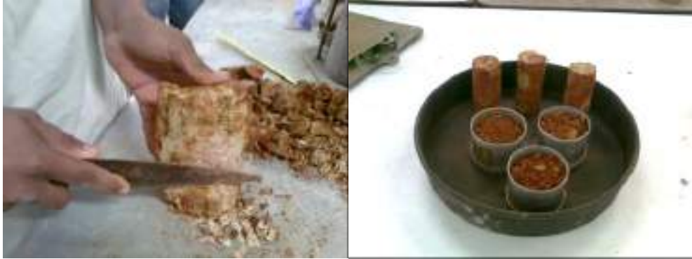
Image 2. Processing of specimens for the triaxial test
