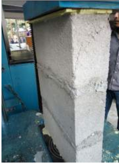
Image 4. Compression test in block piles
