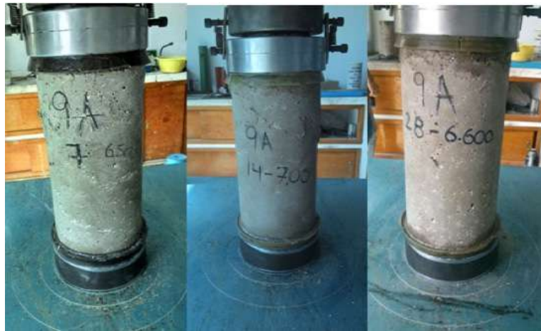
Image 10. Uniaxial compression cylinder test. Source: Own elaboration
