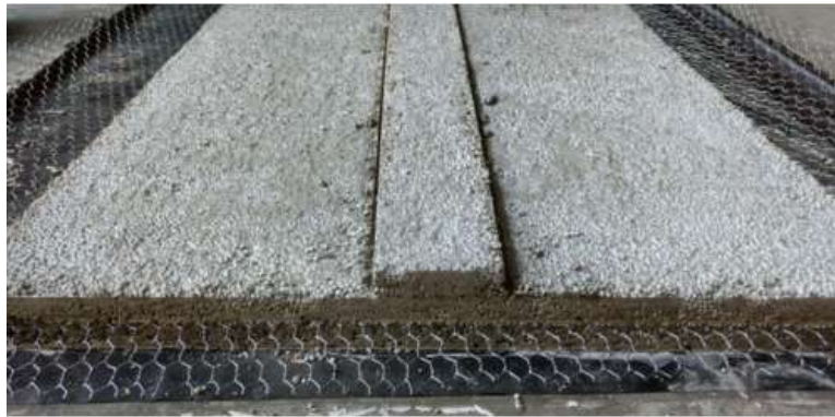
Image 3. Recycled concrete panel prototype of 110*60*5 cms, with a bump of 10*2 cms. Source: Romero and Laguna (2017)
