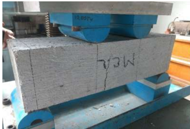
Image 11. Bending beam test. Source: Own elaboration
