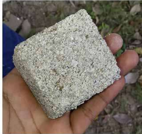
Figure 4. Mortar with 80% sand replacement by the crushed glass (Mv*80). Source: Own elaboration
