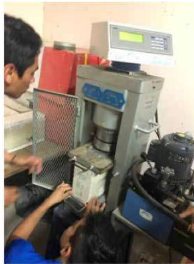
Image 1. Concrete block compression test. Source: Own elaboration
