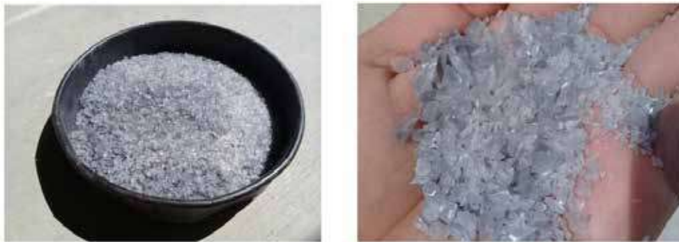
Figure 2. Crushed glass used in mortar mixtures. Source: Own elaboration
