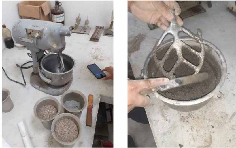
Figure 3. Mixing of conventional mortar. Source: Own elaboration
