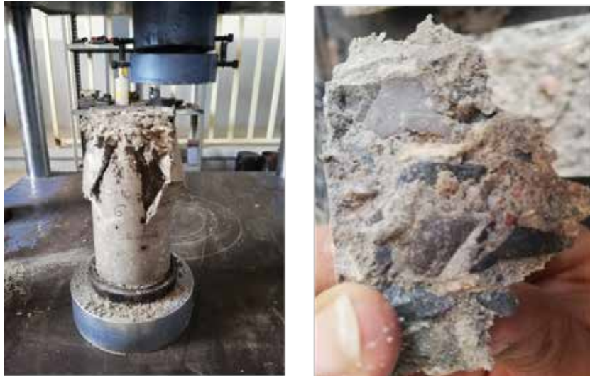
Figure 11. Cylinder subjected to compression. Source: Image taken in the laboratory
