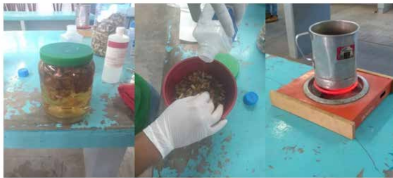
Figure 5. Absorption and density tests in cigarette butts. Source: Image taken in the laboratory
