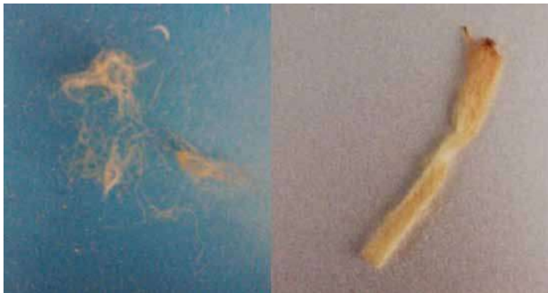
Figure 4. Strands obtained after shredding the butts. Source: Image taken in the laboratory
