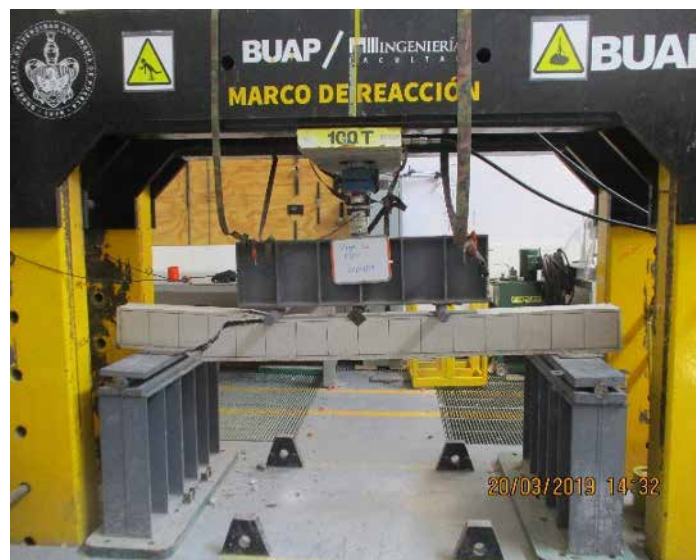
Figure 4. Failure in beams, collapse by shear: beam 4. Source: Own elaboration
