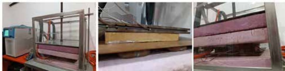
Figure 10. Enabling Wood Panel on Hot Plate Equipment (EPCG)
