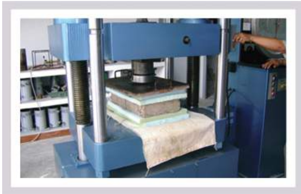
Figure 3. Compression test of the adobe parts (Ovando Ruíz de la Cruz and Castellanos, 2010)
