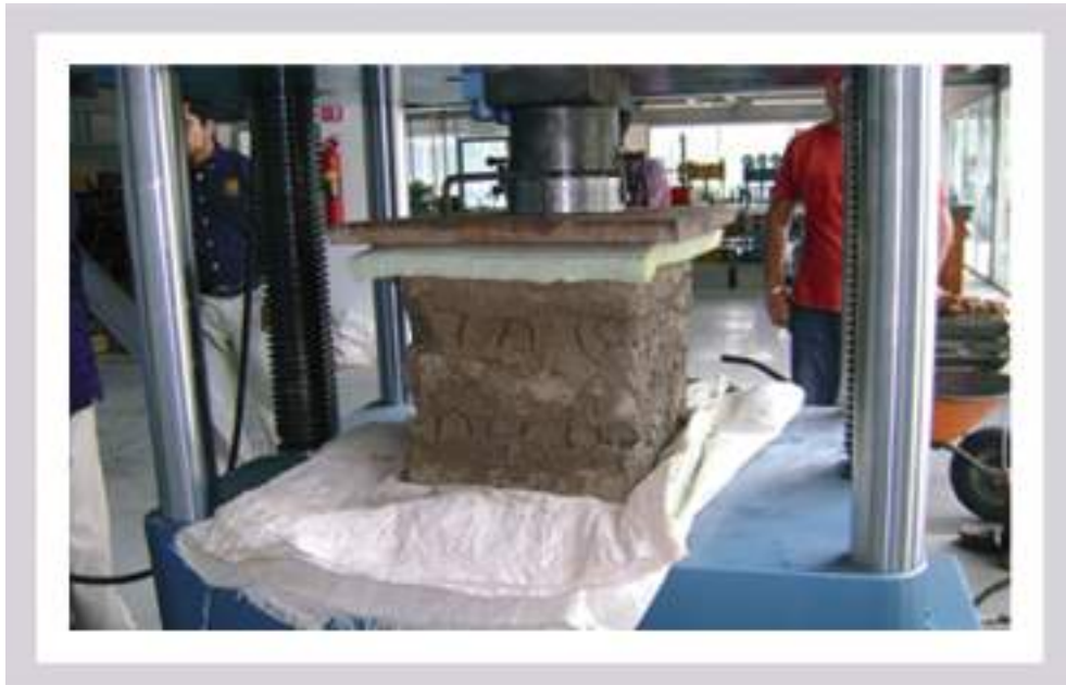
Figure 5. Compression test of adobe stacks (Ovando de la Cruz y Ruíz Castellanos, 2010)
